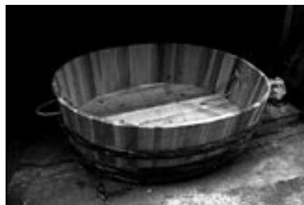
The taraibune, or tub boat, built by the author and Koichi Fujii in 1996. Tub boats reflect Japanese cooperage, with some subtle differences. They are oval rather than round, which makes them track better at sea. About 200 of these boats are still used for fishing on Sado Island.
